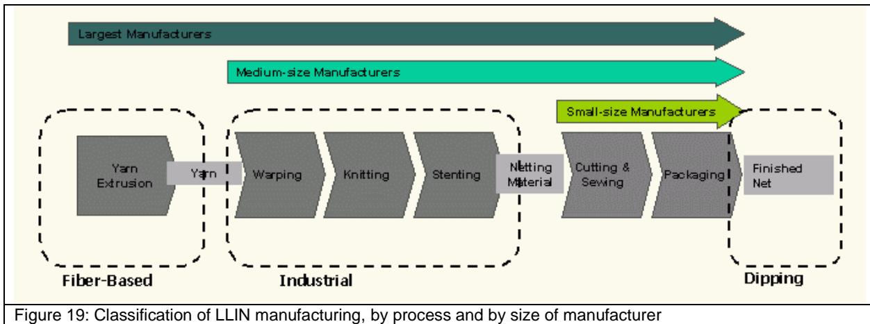
Figure 19: Classification of LLIN manufacturing, by process and by size of manufacturer
