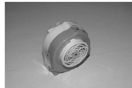
Figure 1 A portable battery-powered blower that holds 0.6% transfluthrin or 0.6% metofluthrin granules in a cartridge (45 mm in diameter). (A) Vapor outlets, (B) cartridge.
