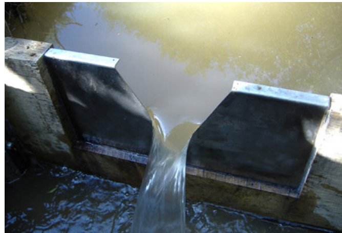
V notch for water use estimation
